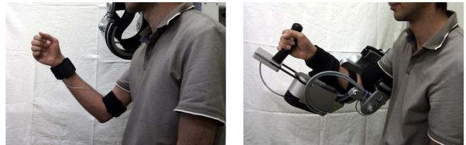
Fig. 1: Experimental Setup in 'Free Reaching' (left) and 'Robot Reaching' (right) conditions. Black straps shown in 'Free reaching' hold lightweight magnetic sensors.
